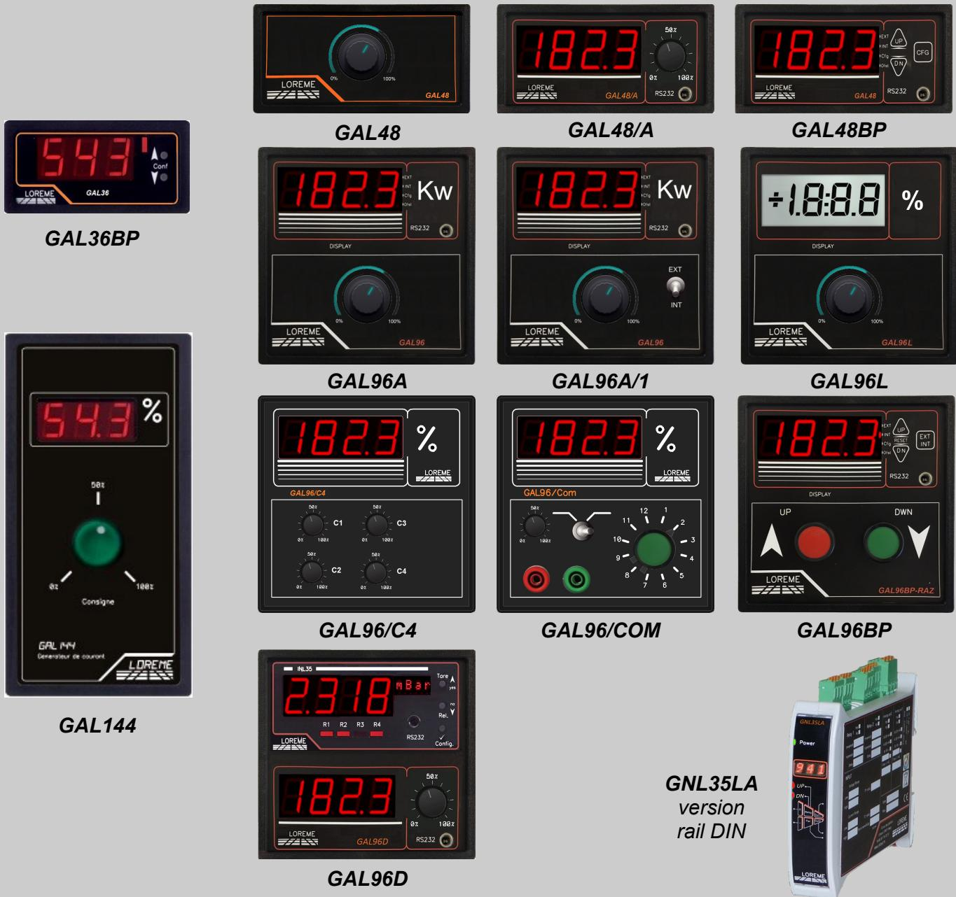
This setpoint generators provide an analog output signal (0... 4... 20mA or 0... 1... 5... 10V), enable to manually drive a machine or an installation. Some version allows to switch between an external setpoint (provide by a PLC, control unit, ...) and the local setpoint.
