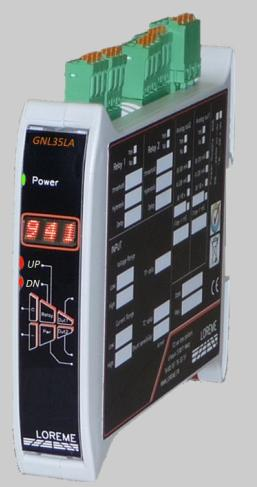
The GNL35LA is a DIN rail mounted setpoint generator with push buttons setting. Fully configurable by front face. Its universal power supply can be Ac or Dc, from 20 to 265V.
