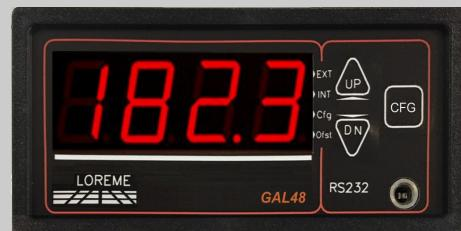
The GAL48BP is a setpoint generator with digital setting. It also allows the display of an external analog input to control the setpoint feedback for example. The display value (setpoint or measure) can be selected with the pushbutton.
