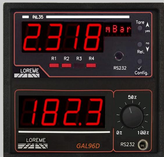
The GAL96D is a setpoint generator, allowing the simultaneous display of the local setpoint as well as an external analog measurement. Both functions are programmable and available in a wide range of auxiliary power supplies.
